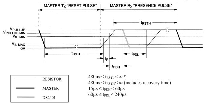
\* In order not to mask interrupt signaling by other devices on the 1-Wire bus,  $t_{RSTL} + t_R$  should always be less than 960 $\mu$ s.
